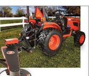
Spring mowing arm allows the cutting head to automatically turn away from poles, trees and other obstacles Comfortably mows all weeds and long grass around fencing from the
